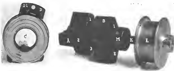
Fig. 3.—The Strip Copper Winding and the Inductors.
